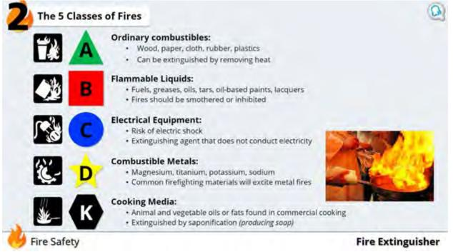
Class K extinguishers may require specific training, including when they should be used or not used. For example, the extinguishing agents in many Class K extinguishers are electrically conductive and should only be used after electrical power to the kitchen appliance has been shut off.
